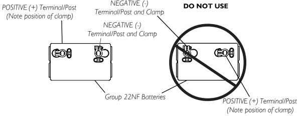
FIGURE 11.6 Connecting Battery Cables
